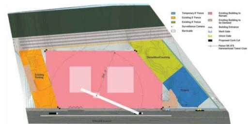
Figure 14 Site plan with crane radius
