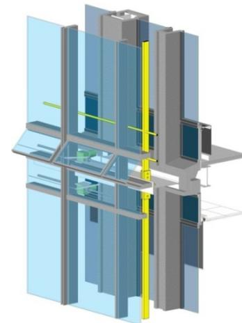
Figure 5 Curtain wall digital mock-up
