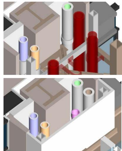
Figure 12 Detailed demolition and installation phasing of facade elements
