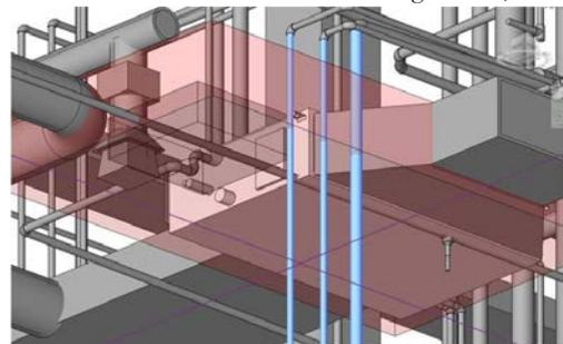
Figure 11. Transparent red volume indicates clearance zone required for mechanical maintenance
