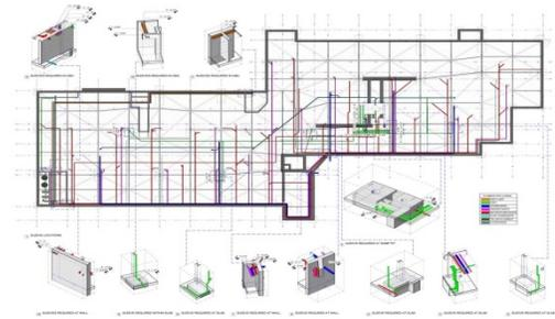
Figure 8 Color-coded plan showing pipe embed locations
